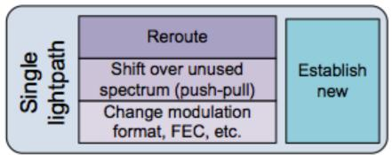
Possible actions to re-act against a degradation/failure are included in the Library of Control Primitives:
