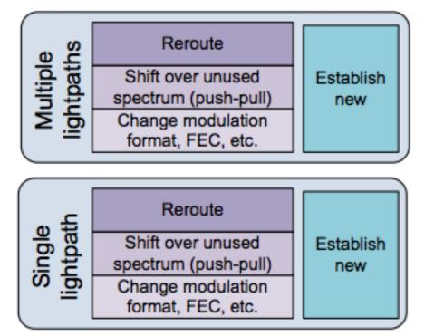
Possible actions to re-act against a degradation/failure are included in the Library of Control Primitives:
